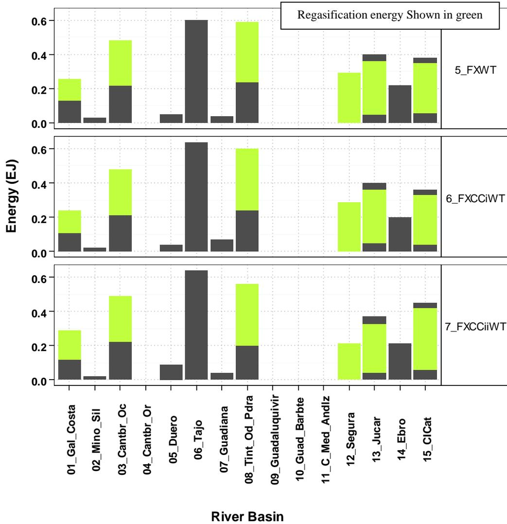
Figure 8: Comparison of Distributed Energy Output "FXWT", "FXCCiWT" & "FXCCiiWT"
